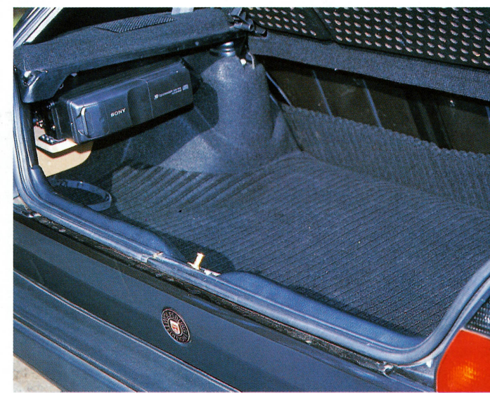
Boot is not as deep as the standard Mk2 because of the car's 4WD mechanics
